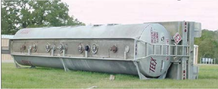
Figure 3.2: Overturned MC-306/DOT-406 Cargo Tank
