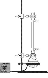
Reflux Column on Triple Neck Flask
