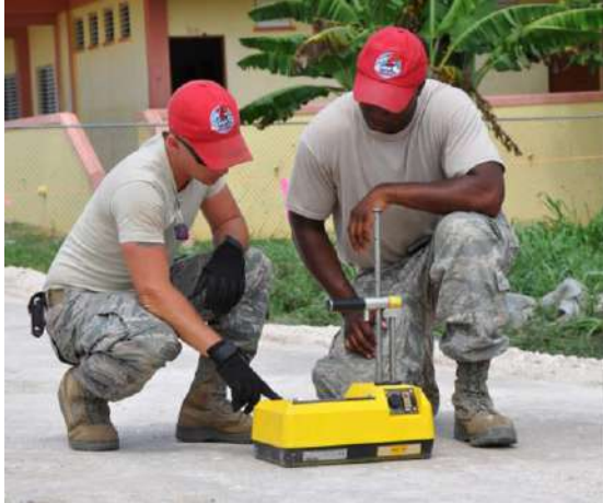
A density gauge used to measure foundation base compaction (Source: U.S. Department of Defense) and different nuclear density gauges (Source: American Portable Nuclear Gauge Association).
