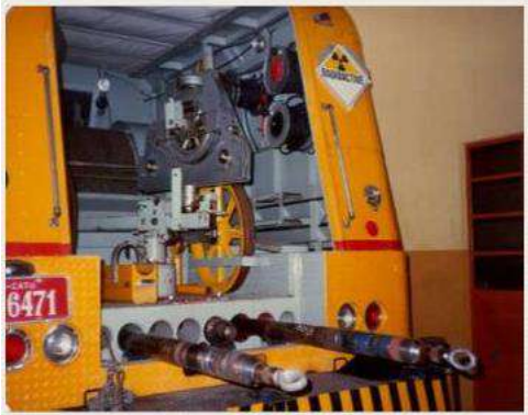
Well loggers on truck (Source: IAEA)
