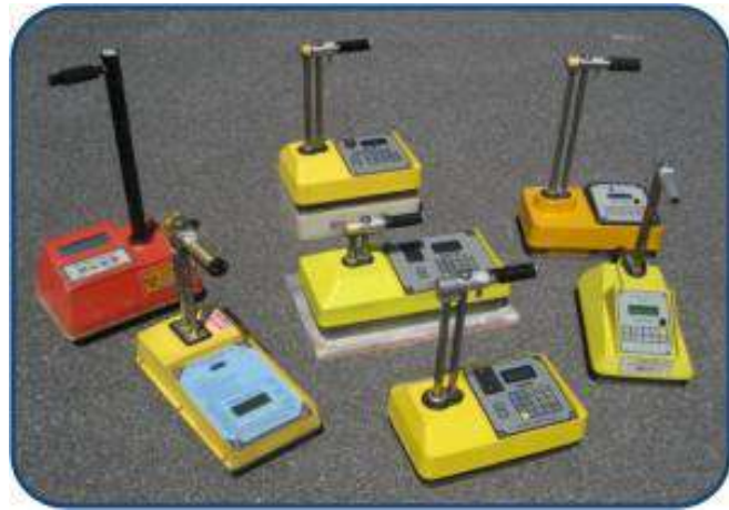
A density gauge used to measure foundation base compaction (Source: U.S. Department of Defense) and different nuclear density gauges (Source: American Portable Nuclear Gauge Association).
