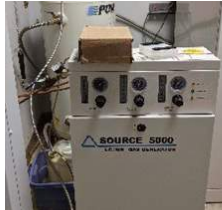
Images: local compressor supporting nitrogen generator
